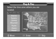
9. Press the ▲ or ▼ button to highlight the time zone for your local area (and to move the highlight to the appropriate time zone on the map of the United States). Press the ENTER button.
